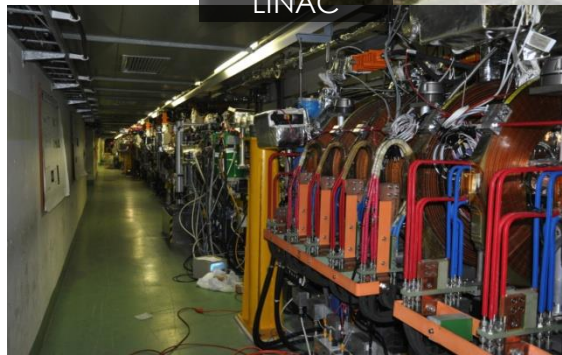
DRIVE BEAM LINAC
