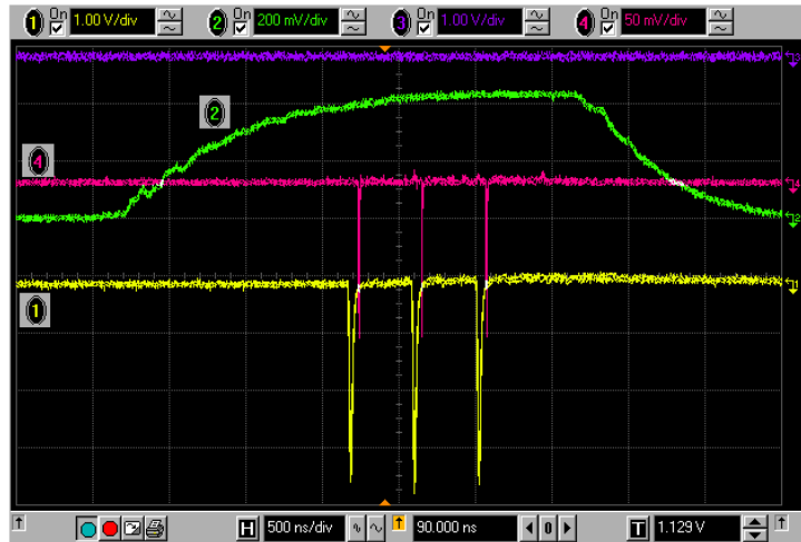
Figure 3: First CTF3 beam multi-pulse: 1-ECM signal, 2-Buncher loop, 4- WCM26 signal.
