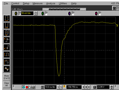
Figure 7: ECM signal for the nominal current in the gun.
