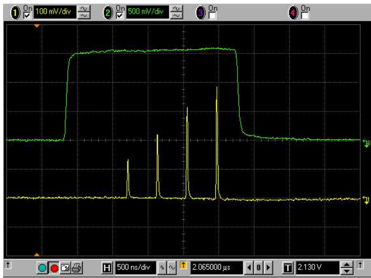
Figure 2: Visualization of the signal from the beam position monitor HR.UMA83 (bottom) turn after turn while the bunch train combination is performed. The RF pulse in WL.MDK33 is also shown (top).
