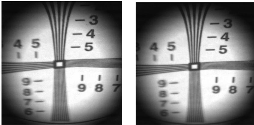
Figure 5: Sample Image observed with a standard setup consisting of two achromatic lenses (left) and with the second lens replaced by a fused silica lens (right).
