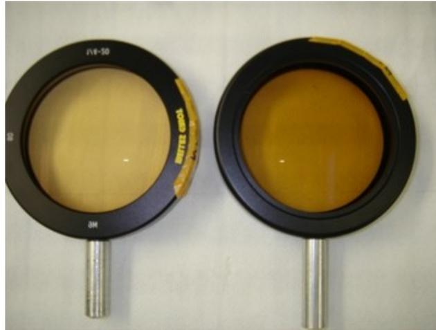
Figure 4: Achromatic lenses installed at CL.MTV1030 after three weeks of operation. The second lens (which is located at the same height as the beam pipe) is shown on the right.
