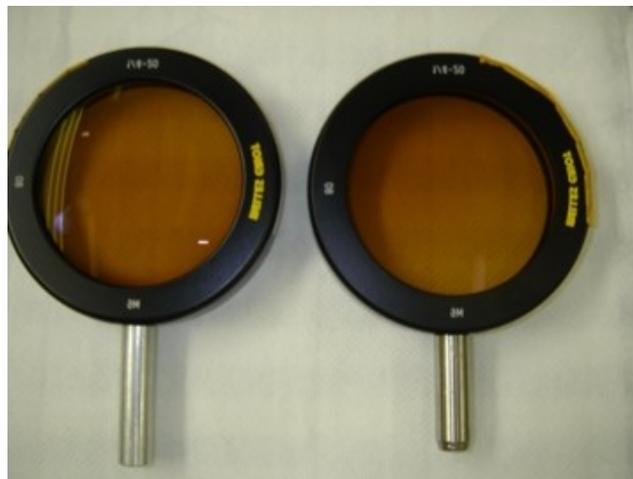
Figure 3: Achromatic lenses installed at CTS.MTV1040 after two years of operation. The second lens (which is located at the same height as the beam pipe) is shown on the right.
