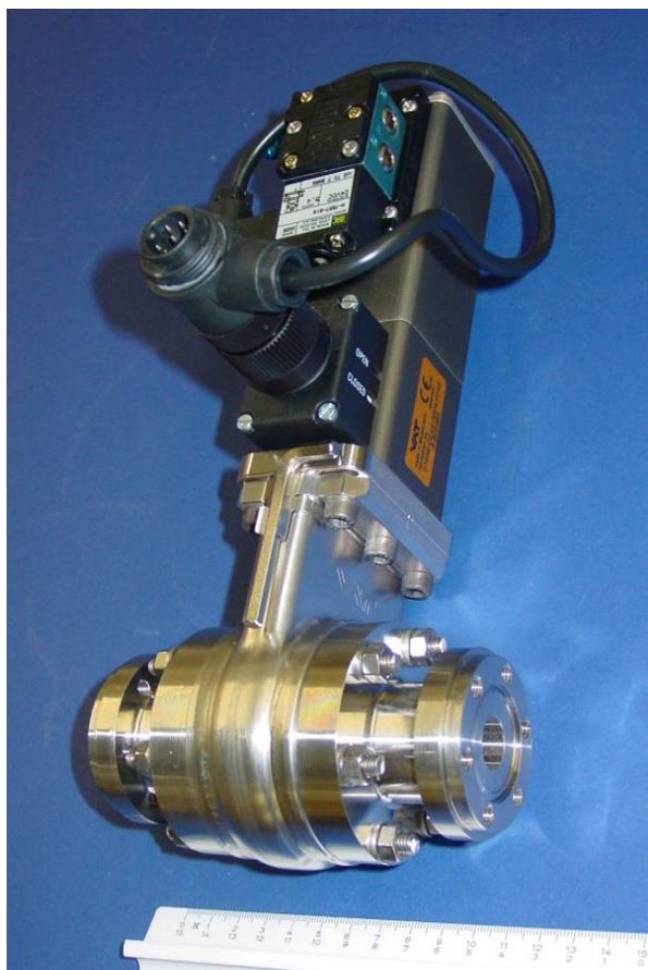
Figure 4: Fully assembled 30 GHz compact dual-mode rf waveguide vacuum valve.
