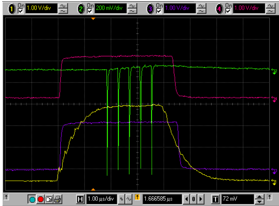
Figure 1: Five pulses inside the RF pulses of MDK25 (bunching system), MDK27 and MDK31.
